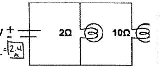
d. Use the total current and the total voltage to calculate the total resistance of the circuit.
